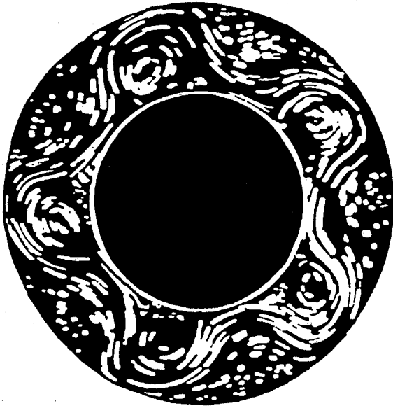
Fig. 1. A streak photograph of trajectories of the suspended particles at a depth of 0.5 cm below the upper surface by exposing the film for 2 seconds in a camera mounted on the rotating apparatus, taken from Hide and Mason (1975). Working fluid is a water-glycerol solution. The size of the annulus is b - a = 4.64 cm and d = 13.5 cm. Rotation rate is 3.22 rad/s and the thermal Rossby number is 0.118.
